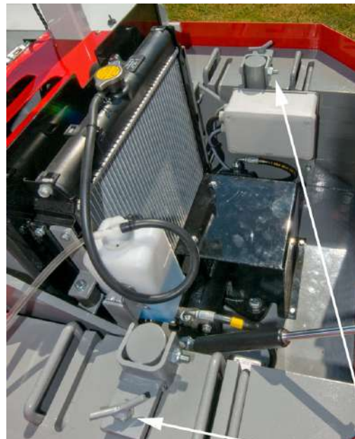
Figure 5.13 | Prins Sprinter ballast plate securing components
