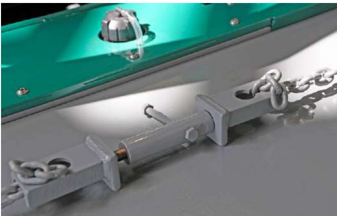
Figure 5.13 | Prins Sprinter ballast plate securing components
